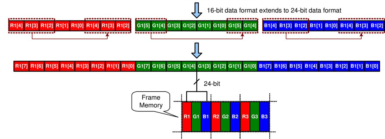
Write data for 18-bit RGB interface bus width set is shown below.
