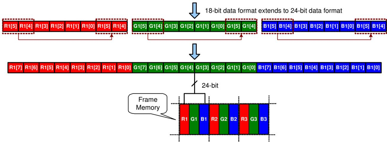
Write data for 24-bit RGB interface bus width set is shown below.
