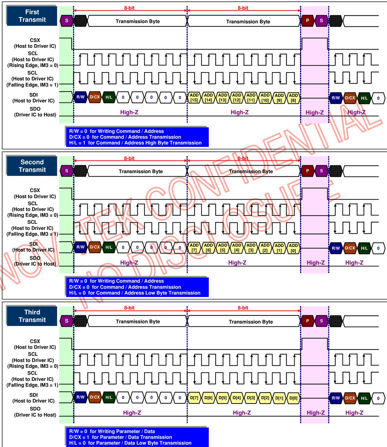
**Fig. 5.1.5 Serial bus protocol for register write mode**
