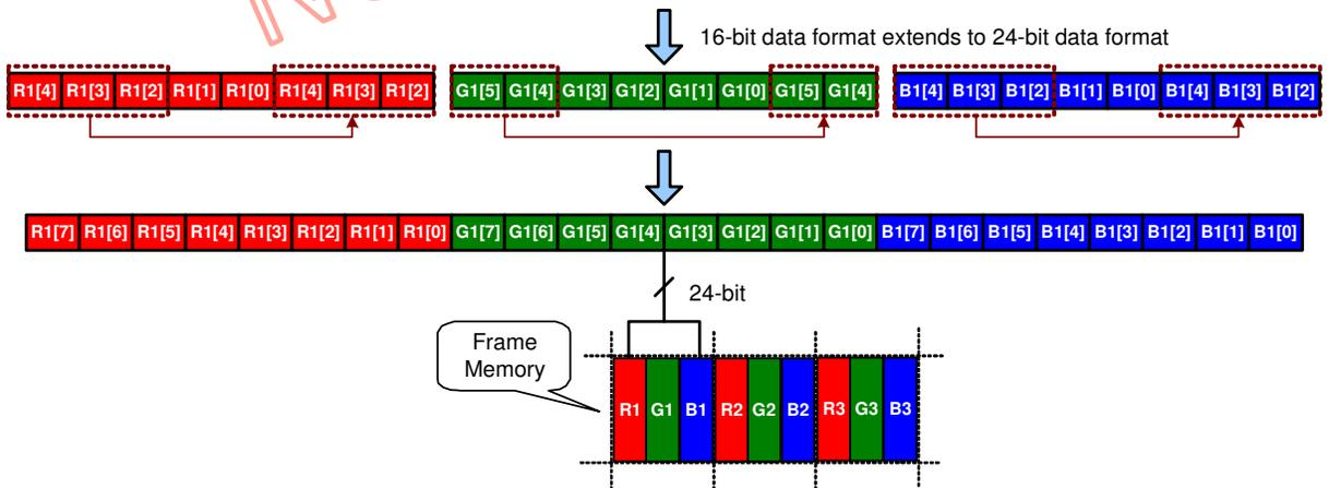
1. In one transfer (D15 to D0), 1 pixel data transmitted with the 16-bit color depth information.
