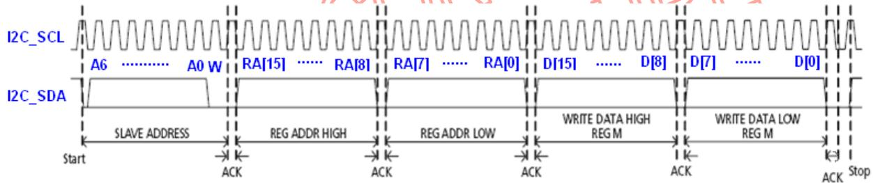
**Fig. 5.2.3 Register Writing Timing of I2C Interface**
