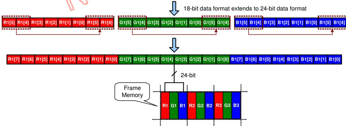
1. 3 times transfer is used to transmit 2 pixel data or 2 times transfer is used to transmit 1 pixel data with the 18-bit color depth information.
