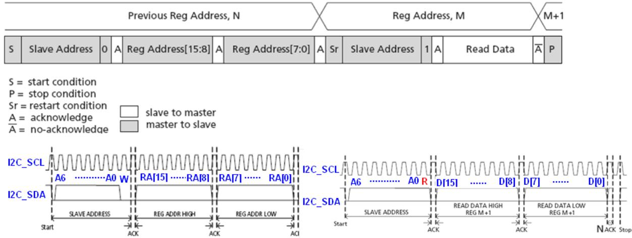
**Fig. 5.2.4 Register Reading Timing of I2C Interface**
