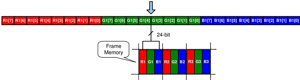
1. In one transfer (D23 to D0), 1 pixel data transmitted with the 24-bit color depth information.
